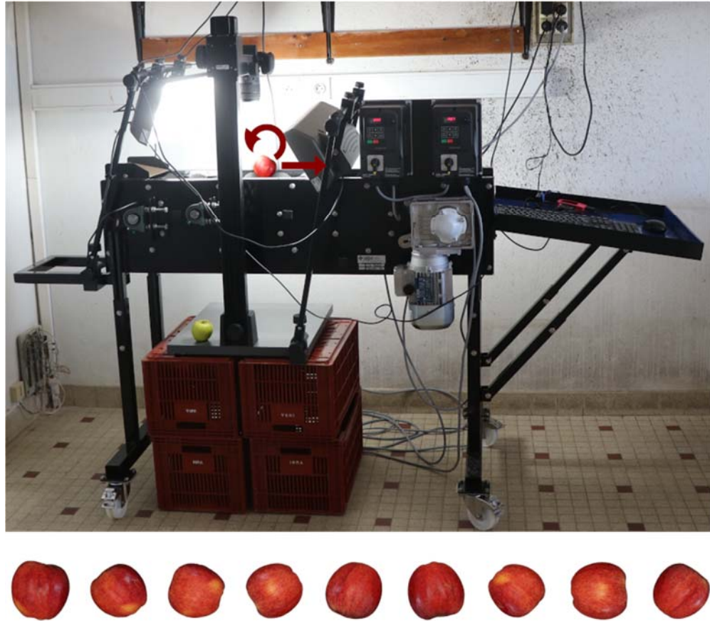
Figure 1. Acquisition system. Upper panel: Machine equipped with a conveyor belt, used for the acquisition of images of apples with a high surface coverage. Lower panel: view of the acquired images of apples after segmentation from the background.
